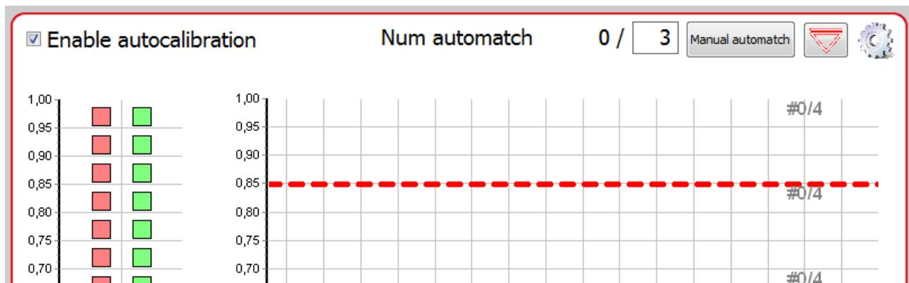
The **step one** consists driving in petrol mode, the system acquires samples in the Injection-time/Map space. The vehicle driver, driving the vehicle both at idle and on-road, must try to cover as much red dots as he can, until a red line is drawn. In this activity the PC software ease the acquisition suggesting which area still needs to be covered, or deleting mistaken samples.
