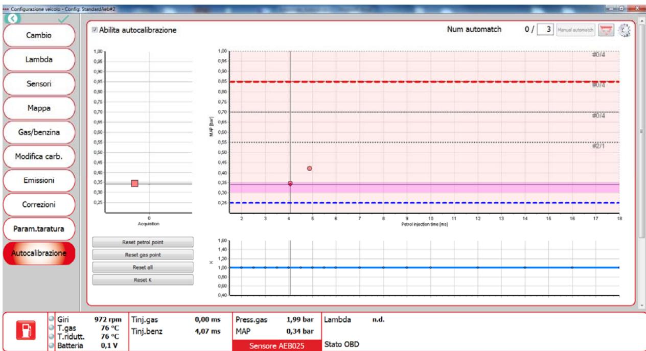
Step one can be concluded as soon as the red line is plotted, but optionally the driver can refine the acquisition continuing the petrol drive.
