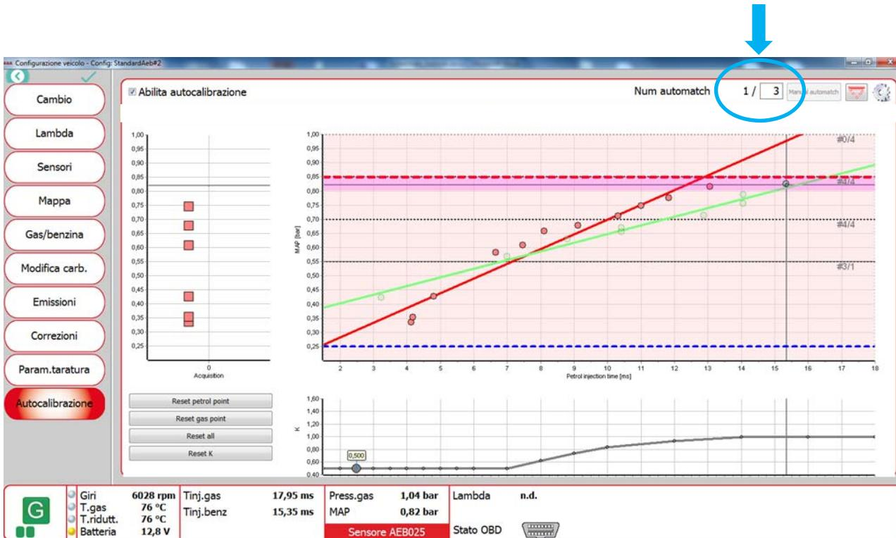
The system acquired the green line the last time, the autocalibration is ended
