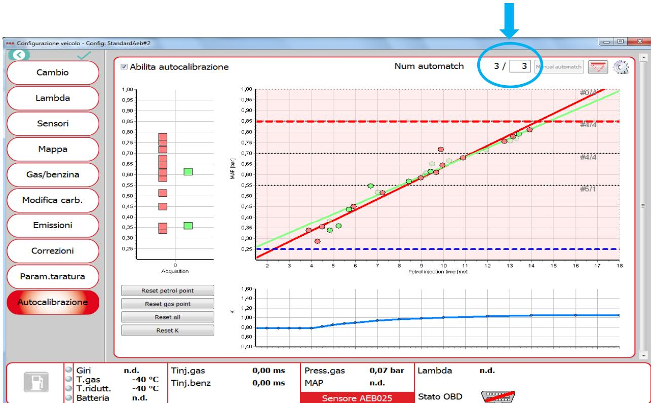
The procedure finishes as the number of automatch reaches the required number of executions; the autocalibration output is K Vector (blue line) different from the usual K map.
