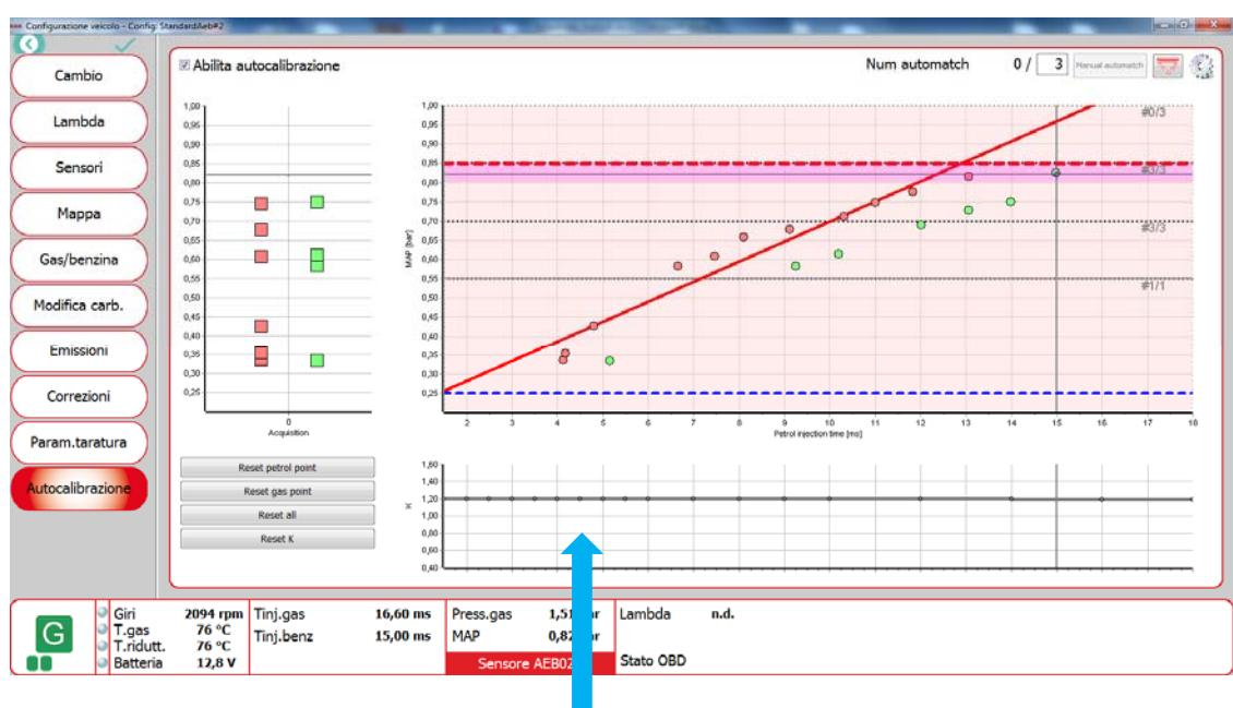
In this example after the first automatch the maximum correction is  $+20\%$  also if should be  $+40\%$
