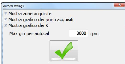
If during the autocalibration the rpm will exceed this threshold of rpm, in petrol mode or in gas mode will appear a Warning
